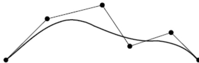
Quasi-uniform B-Spline curve of degree 3
